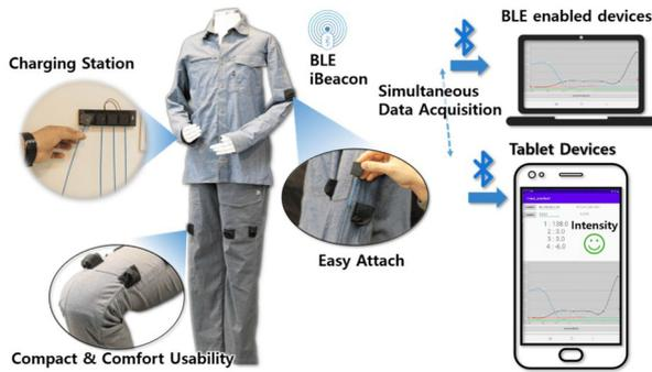
Fig. 1. Schematic of proposed motion-sensing smart work suit system comprising a traditional working suit, wireless bend sensing module, charging station, and monitoring devices.
