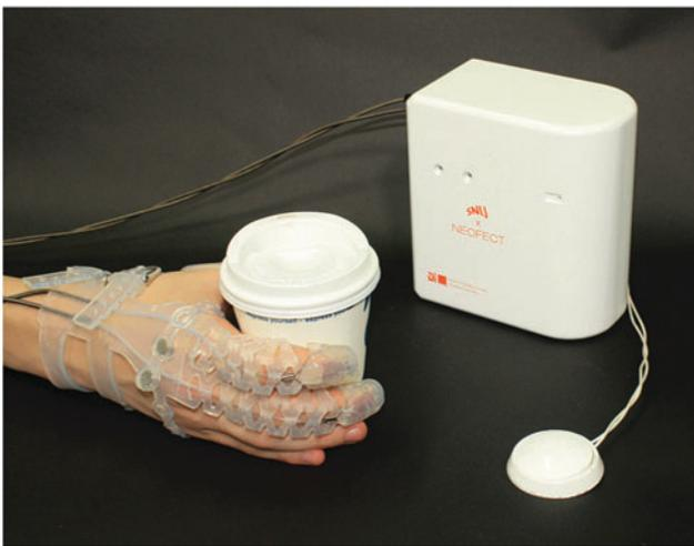
**FIG. 1.** EGP consists of a soft polymer glove, wire sheaths, and an actuation system and a freestanding intention button that users press to actuate the glove. EGP, Exo-Glove Poly.
