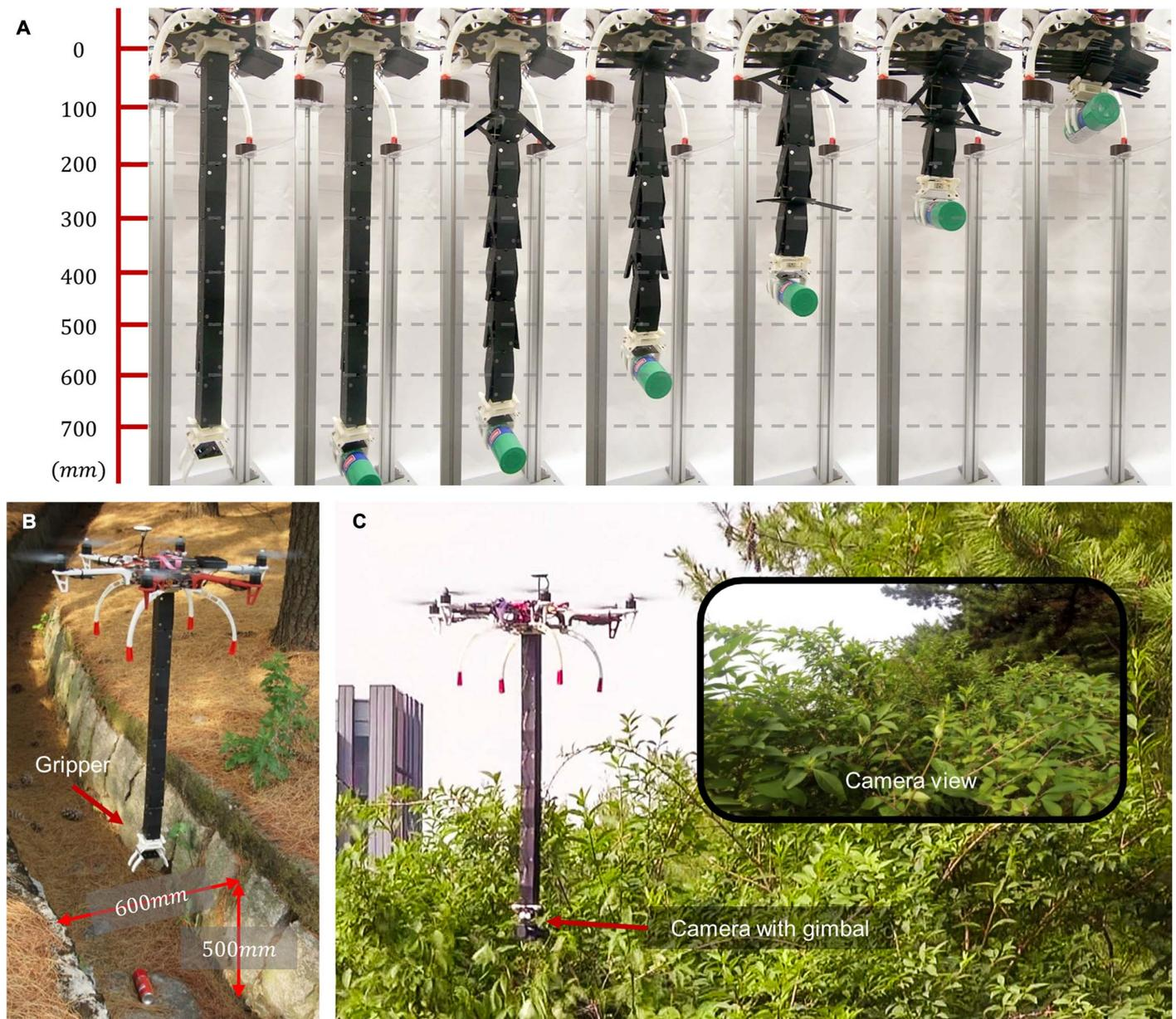
**Fig. 7. The foldable robotic arm with seven modules assembled in series. (A)** Stills from a movie that shows folding process of the arm. **(B)** Foldable arm picking up objects with its gripper at the bottom of a 500-mm-deep ditch. **(C)** A camera and a gimbal were attached to the arm and filmed between branches.
