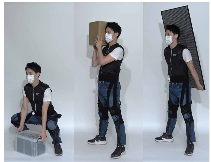
Movie 1. Overview of unpowered soft exosuit with body-powered variable impedance. This video summarizes the principles and performance of the developed exosuit.
