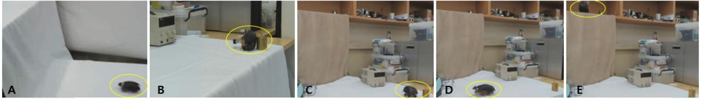
Fig. 16. Reaching target place through integrated jumping–crawling and self-righting. The robot (a) overcomes an 0.90-m obstacle, (b) and (c) stands upright itself, and (d) maneuvers toward the target. (e) Robot jumps again and finally, reaches the target.
