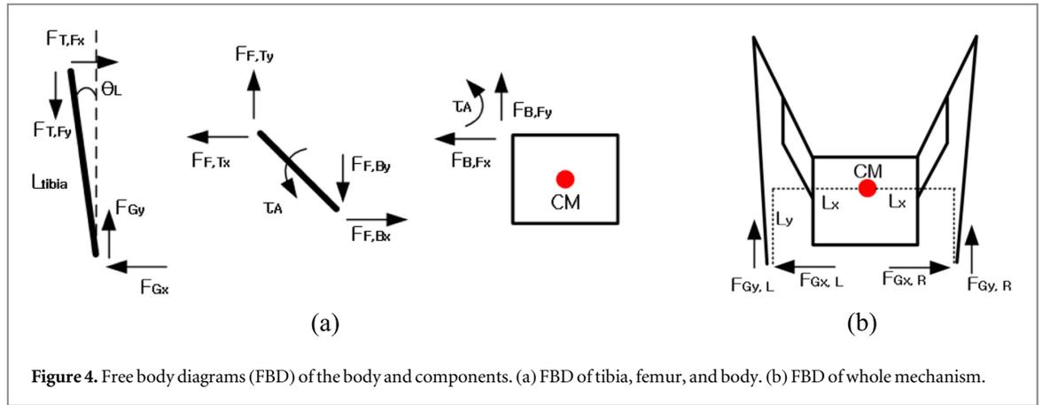
Figure 4. Free body diagrams (FBD) of the body and components. (a) FBD of tibia, femur, and body. (b) FBD of whole mechanism.
