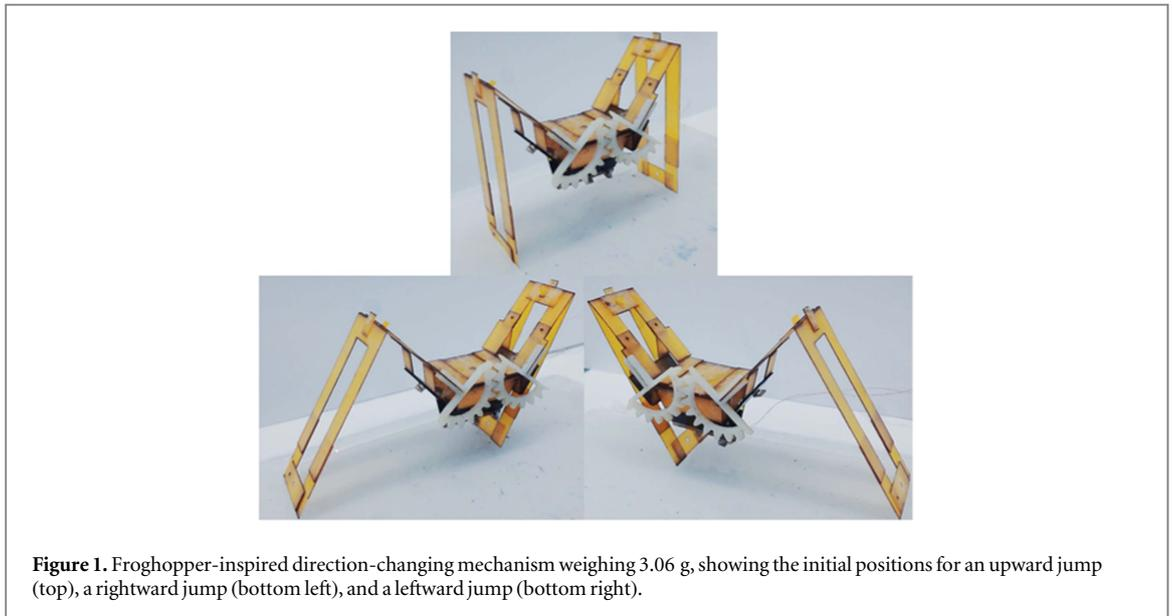
**Figure 1.** Froghopper-inspired direction-changing mechanism weighing 3.06 g, showing the initial positions for an upward jump (top), a rightward jump (bottom left), and a leftward jump (bottom right).
