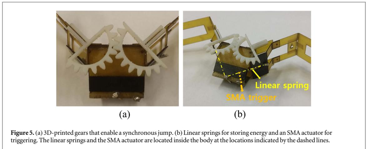
**Figure 5.** (a) 3D-printed gears that enable a synchronous jump. (b) Linear springs for storing energy and an SMA actuator for triggering. The linear springs and the SMA actuator are located inside the body at the locations indicated by the dashed lines.
