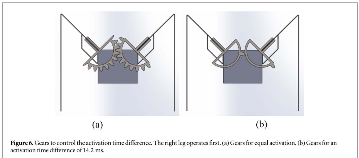
**Figure 6.** Gears to control the activation time difference. The right leg operates first. (a) Gears for equal activation. (b) Gears for an activation time difference of 14.2 ms.
