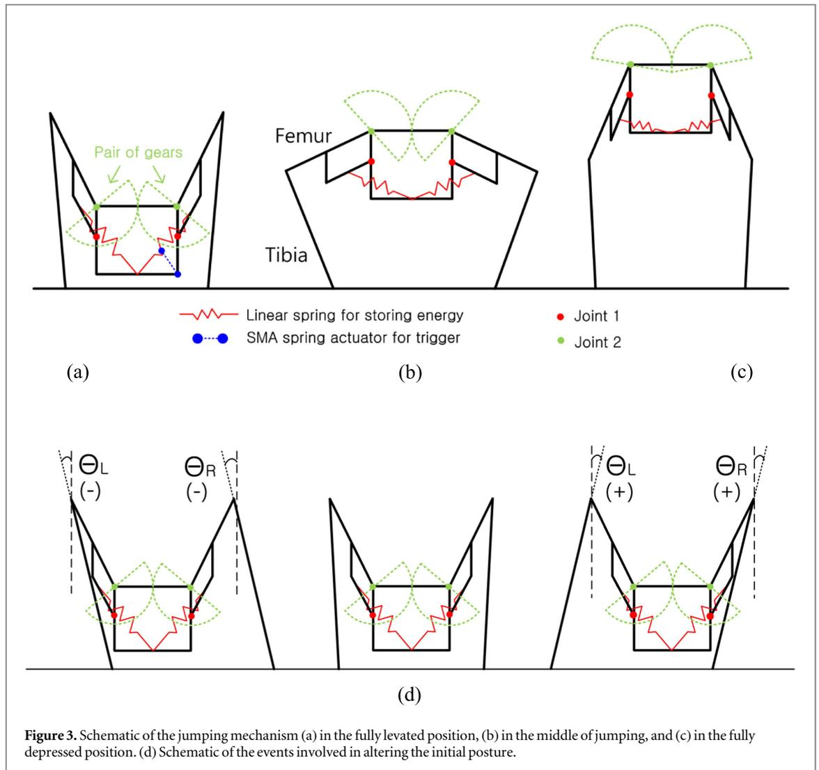
**Figure 3.** Schematic of the jumping mechanism (a) in the fully levated position, (b) in the middle of jumping, and (c) in the fully depressed position. (d) Schematic of the events involved in altering the initial posture.
