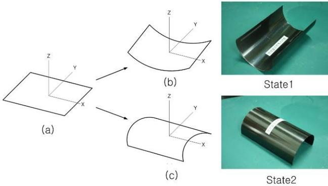
Fig. 3. [90/0] Bi-stable composite structure reference coordinates.
