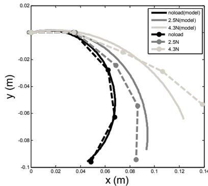
Fig. 10. Plot of numerical result (solid line) and experimental result (dashed line) at state 2 of the bi-stable structure.
