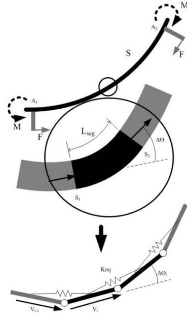
Fig. 6. Segmented linkage model for composite flexure.
