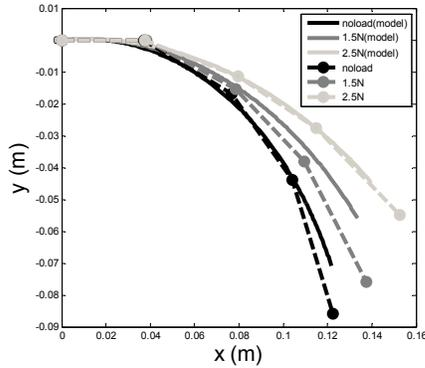
Fig. 9. Numerical result (solid line) and experimental result (dashed line) plot at state 1 of the bi-stable structure.
