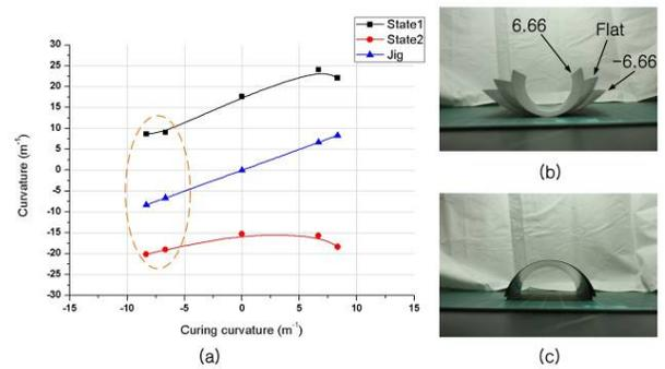
Fig. 4. (a) CFRP laminate curvature from various curvature jig plate curing process.(unclear: too long) orange dashed circle inside region shows that state one has small curvature and state two has large curvature.
