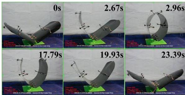
Fig. 12. Flytrap robot performance sequences. Upper part shows the closing motion and lower part shows the opening motion.
