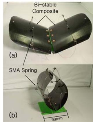
Fig. 1. Flytrap robot with SMA spring actuator. (a) is opened state and (b) is closed state.
