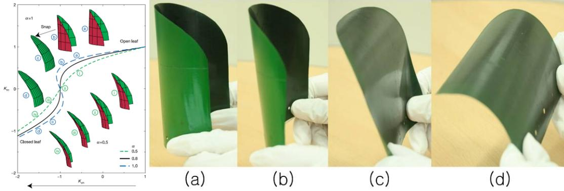
Fig. 2. The flytrap's smooth-snapping transition in leaf closure diagram (far left figure) [1]. Applying bending moment by fingers, CFRP composite snap-through progress sequence from (a) to (d). Snap-through occurs between (b) to (c) [2].
