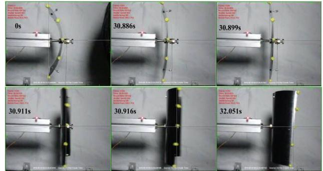
Fig. 8. Snap-through sequences of the bi-stable CFRP structure. Attached bold rod distance was 130mm and the moment arm was 15mm. The snap-through time was about 17ms.
