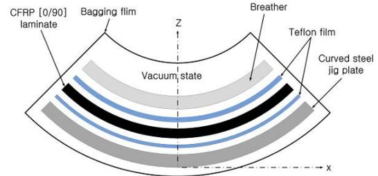
Fig. 11. The scheme of curing materials layup. In the notation [0/90], 0 layer means that the angle between the CFRP fiber direction and the jig plate curvature axis is zero.
