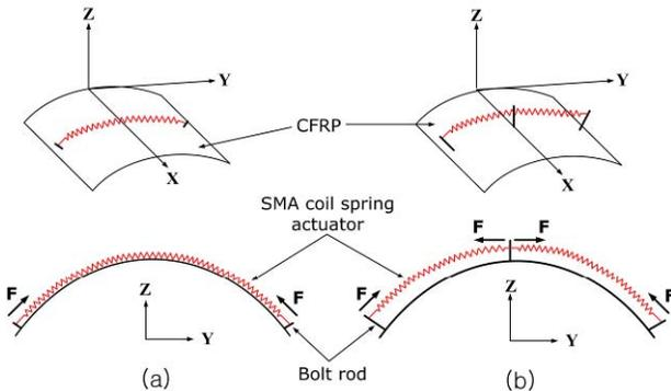
Fig. 5. Comparative scheme of attachment of SMA coil spring actuator on the bi-stable CFRP structure. (a) Small bolt rods induce small bending moment. Also the middle of spring contacts the CFRP surface. (b) The structure has three long rods which induces a large bending moment. The spring is now separated from the CFRP surface.
