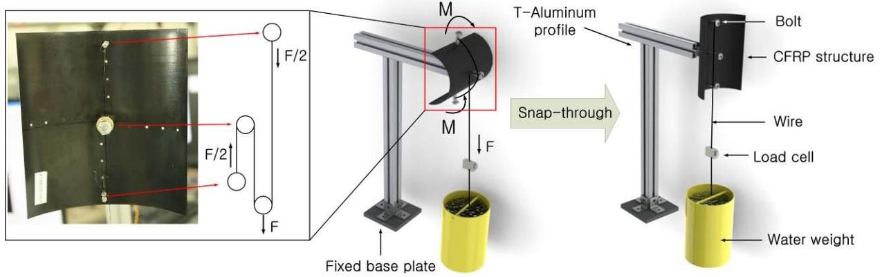
Fig. 7. Description of snap-through force measurement experimental setup. As the water weight increase, wire tension increases and bending moment at the bolt connected between wire and CFRP structure also increase. When the load reaches at critical point, CFRP structure changes its configuration from state 1 to state 2 via snap-through.  $M$  indicates bending moment and  $F$  indicates tensile force due to water weight.
