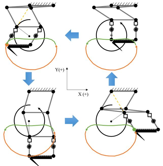
Fig. 6. Schematic diagram of the quick-return leg.
