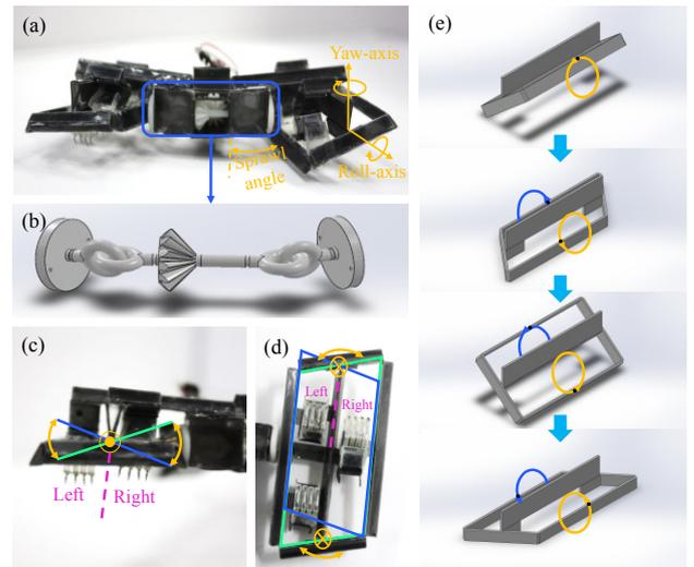
Fig. 3. (a) Components of the transmission system. (b) Shaft with ring-shaped universal joints. (c, d) Rotation about (c) the roll-axis and (d) the yaw-axis. (e) The four different positions of the four-bar linkage, which is composed of eight hinges for an alternating tripod.
