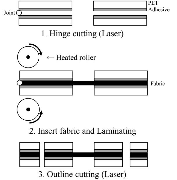
Fig. 8. Facile fabrication using laminating film.
