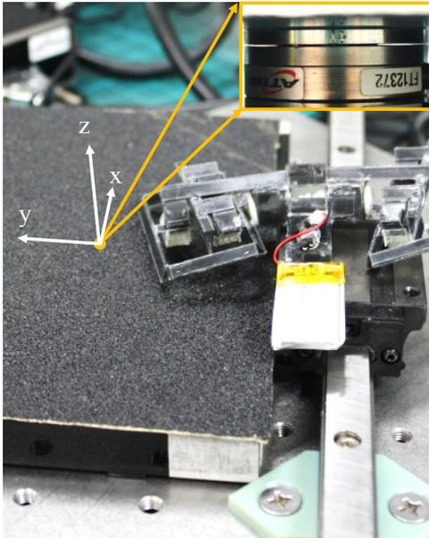
Fig. 9. Experimental setup and the six-axis force/torque sensor.
