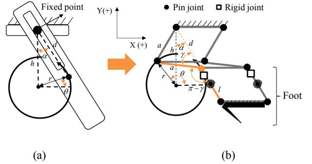
Fig. 5. Design parameters of (a) a conventional quick-return mechanism and (b) a quick-return leg.
