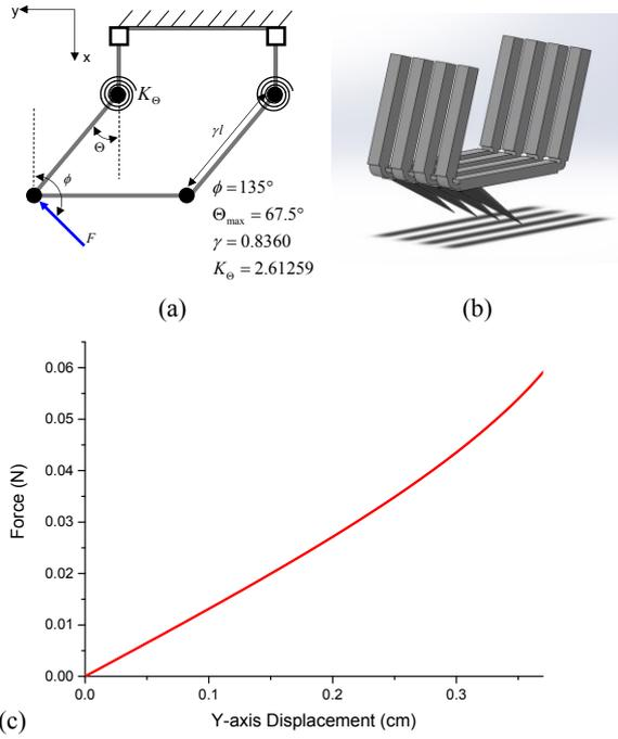
Fig. 4. (a) Spine modeling and numerical data [16]. (b) A compliant foot with four spines. (c) Spine force plotted against deflection.
