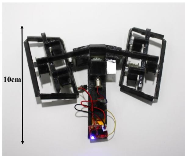
Fig. 1. Small and lightweight climbing platform.
