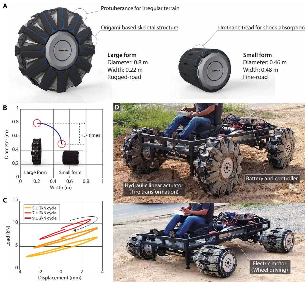
**Fig. 1. Transformable wheel concept and demonstration.** (A) The wheel can be transformed into two shapes according to the road condition. (B) The relationship between the diameter and width of the wheel. (C) The load-displacement response of the wheel in the shape-transition state. (D) We designed a single-passenger vehicle for installation of the transformable wheels. The operation and capacity of the wheels were demonstrated through a field test.
