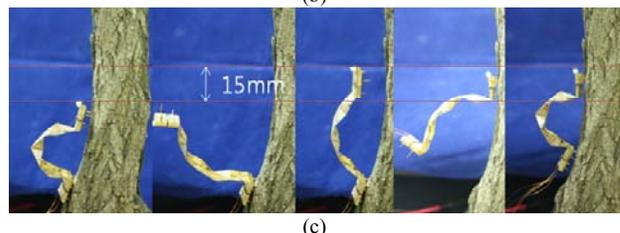
Fig. 11. (a)Steering motion (b)Gripping motion, white shows the compliant gripping area (c)Two anchor climbing motion.
