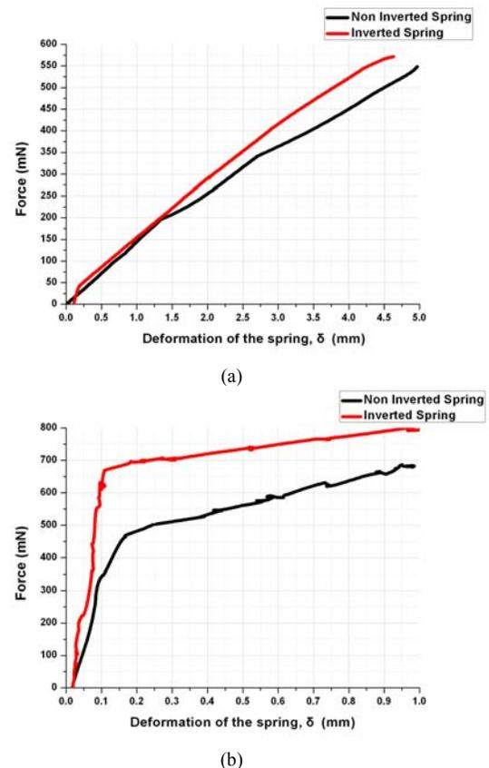
Fig. 8. Force-the deflection curves of Non-inverted and inverted SMA spring Actuator at (a) Martensite and (b) austenite state.
