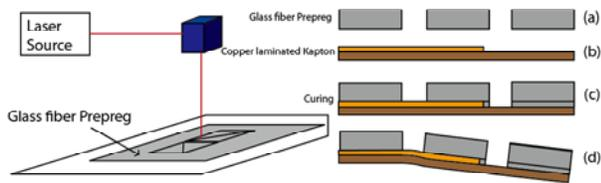
Fig. 9. Overview of the laser micro machining step of the SCM process. (a) Composite prepreg. (b) Thin-film copper laminated polymer are laser cut and etched to make circuit. (c) Curing of the laminae to form segments. (d) finally, circuit embedding structure capable of bending.
