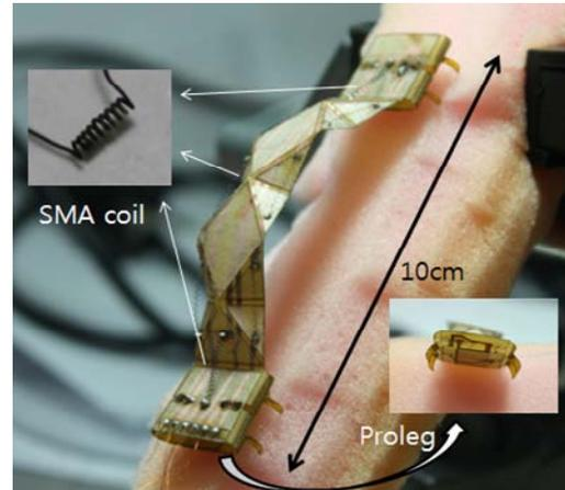
Fig. 1. Omegabot, a biomimetic inchworm robot that can climb vertical wood.
