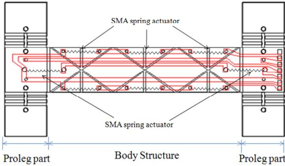
Fig. 2. (a) Exploded diagram of Omegabot. (b) 2-D pattern design of Omegabot. Black line: glass fiber composite prepreg cutting pattern. Red line: copper-laminated Kapton circuit.
