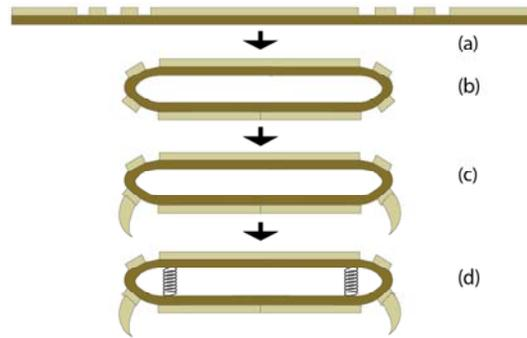
Fig. 10. Artificial proleg fabrication procedure. (a) Cured film of Glass fiber prepreg and Kapton (poly imide) film (b) Bend and make two layer structure (c) Attach the claws (d) Soldering the SMA spring actuator.
