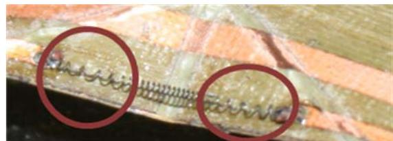
Fig. 6. The drawback of uneven cooling in martensitic transformation.
