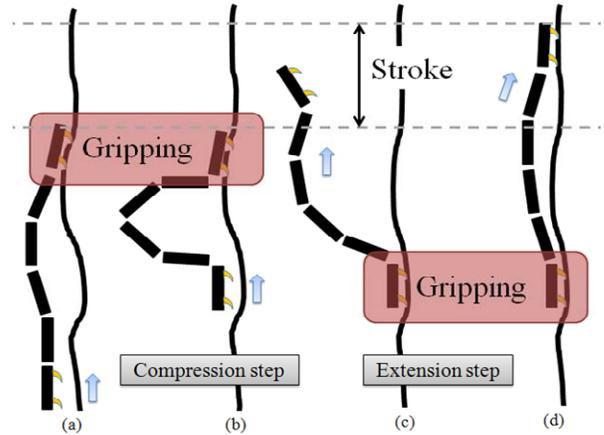
Fig. 5. Climbing procedure of The climbing Omegabot. (a)Head proleg gripping (b)Compression of body frame (c)Tail proleg gripping (d)Extension of body frame.
