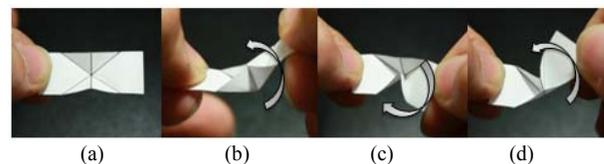
Fig. 3. Paper origami trial version of SCM universal joint. (a) Neutral state. (b) Pitch bending motion. (c)-(d) Yaw bending motions [2].
