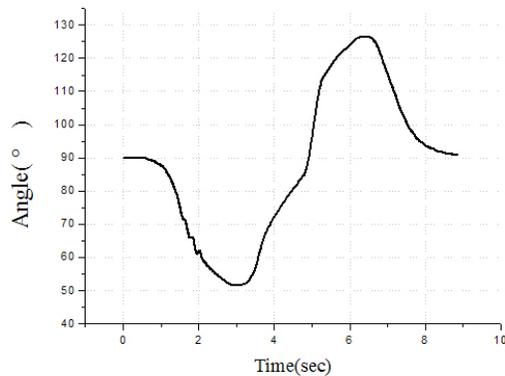
Fig. 12. Steering angle-Time curves of the climbing Omegabot. trajectory is shown in Fig. 12.
