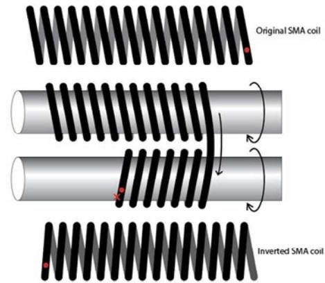
Fig. 7. Inversion of SMA coil actuator by recoiling in the opposite direction.
