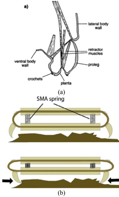
Fig. 4. (a) Transverse section through part of an abdominal segment of a caterpillar showing a proleg [14]. (b) Conceptual design of Omegabot's proleg.
